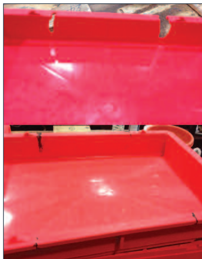
Figure 2: Venting issues in molding a large tote: a short-shot with a gas trap at end of fill (top half of image) and resulting burn marks on part (bottom).
